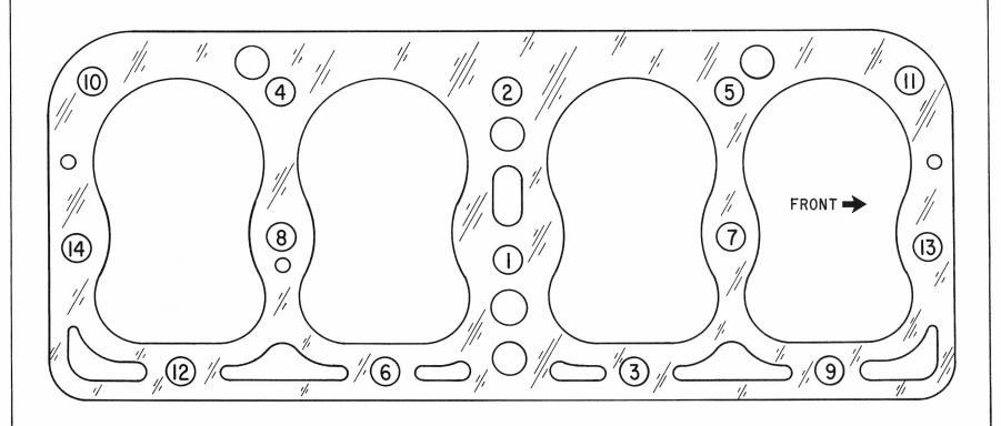
Beginning at cylinder head bolt #1 and moving in numerical sequence to bolt #2, then #3, etc., tighten nuts to final full torque of 50 foot-pounds by following the five steps listed below.
